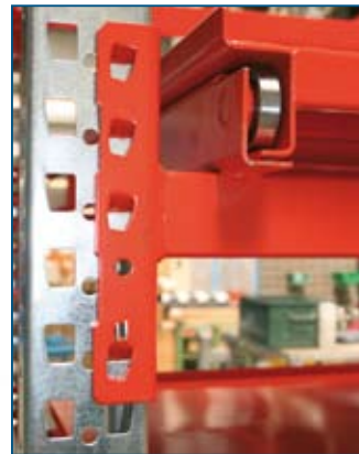
Beam to column and drawers with ball bearing guides.
