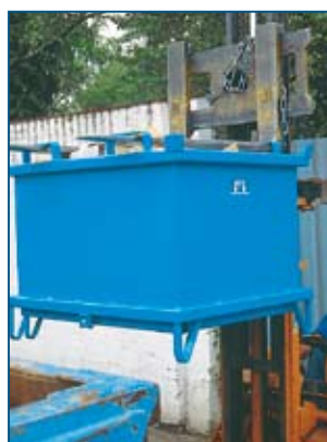
Hinged bottom locks automatically after emptying
