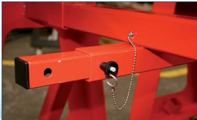
Locking pin with axial lock.
